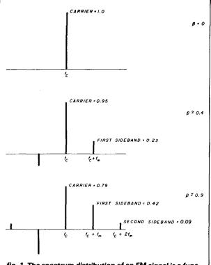
fig. 1. The spectrum distribution of an FM signal is a function of the modulation index  $\beta$  which in turn depends on the amplitude of the modulating (voice) signal. (A) the unmodulated carrier, (B) at a  $\beta$  of 0.4 a single sideband pair is evident with approximately 1/4 of the amplitude of the *un*modulated carrier, and (C) by increasing  $\beta$ to 0.9 a second sideband pair is also apparent. Notice that in both (B) and (C) the carrier power is reduced from its unmodulated value.
